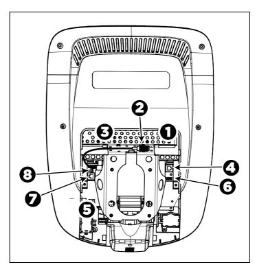
Figure 11: Cable connections, P80 console
